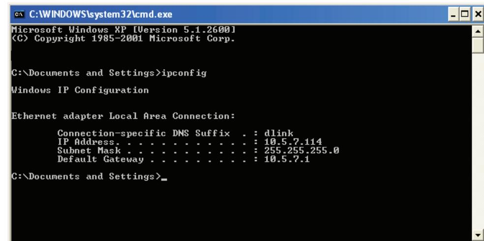
The screenshot shows a Windows XP Command Prompt window titled 'C:\WINDOWS\system32\cmd.exe'. The window displays the output of the 'ipconfig' command. The output shows the following details for the 'Ethernet adapter Local Area Connection':
