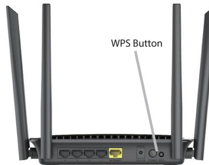
**Step 2** - Within 2 minutes, press the WPS button on your wireless client (or launch the software utility and start the WPS process).
