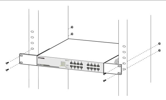
Mount the switch in the rack or chassis using the screws provided with the equipment rack.
