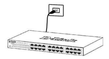
After the switch is powered on, the LED indicators will blink briefly while the system resets.
