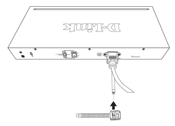
Attach the retainer to the tie wrap
