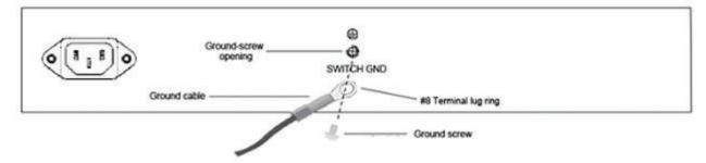
Ground cable, screw and #8 terminal lug rings
