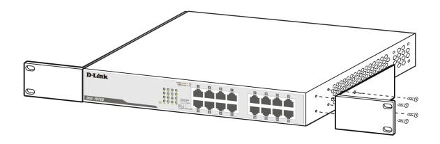
Attach the mounting brackets to the switch
