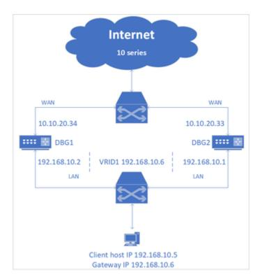
The routers (DBG1 and DBG2) have been configured with the VRRP feature for the LAN interface and are given priority numbers. For example, let's say the priority of DBG1 is 200 and DBG2 is 100. Then, when the client tries to connect to the Internet, it follows the DBG with a higher priority number. Here, it follows DBG1. But, if DBG1 gets disconnected or not reachable, it connects with the second router DBG2, and when DBG1 regains its functionality, it switches to DBG1.
