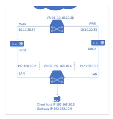
The routers (DBG1 and DBG2) have been configured with the VRRP feature for both the interfaces (LAN and WAN) and are given priority numbers. Then, when the client tries to connect to the Internet, it follows the router with a higher priority number (say DBG1). When the DBG1 WAN is not reachable or disconnected from the topology, it connects to the DBG2 WAN, and when DBG1 WAN gets connected or becomes functional, it again switches to DBG1.
