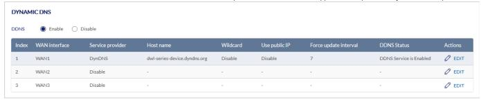
When the DDNS feature is enabled, it is applied to the WAN IP, which is up, and the following fields are displayed in the table:
