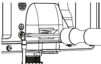
**Figure 12: Attaching the Grounding Wire**
