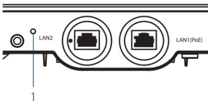
Figure 1: Front Panel LED
