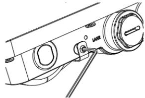
**Figure 10: Securing the Mount Screw**
