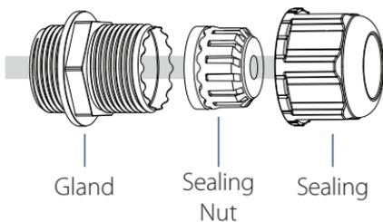
**Figure 4: LAN Port Waterproof Enclosure**
