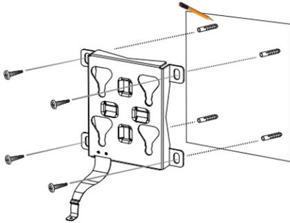
**Figure 7: Attaching the Mounting Plate**
