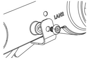
**Figure 9: Attaching the Mount Screw**
