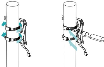
**Figure 5: Attaching the Mounting Plate**
