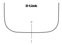
Figure 1: Front Panel LED
