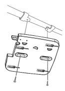
Figure 6: Attaching the Mounting Plate
