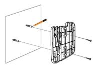
Figure 3: Attaching the Mounting Plate
