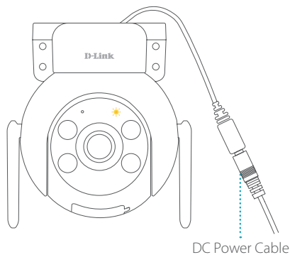
DC Power Cable
