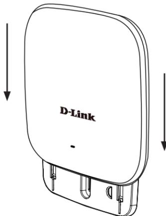
Figure 4: Mounting the Device
