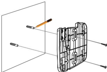
Figure 3: Attaching the Mounting Plate
